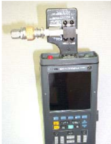
Figure 1.- Scopemeter Pressure Probe Connected to Scopemeter.
